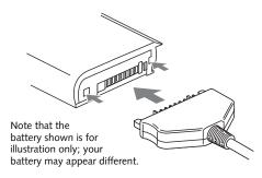
Figure 3. Connecting the battery
